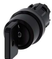
Key-operated switch O.M.R, 22 mm, round, plastic, lock number 73034, black, with 2 keys, 3 switch positions I-O-II, latching, actuating angle 2x45°, 10:30h/12h/13:30h, Key removal I+O+II
