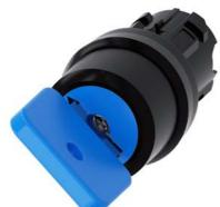
Key-operated switch O.M.R, 22 mm, round, plastic, lock number 73038, blue, with 2 keys, 2 switch positions O-I, latching, actuating angle  $90^\circ$ , 10:30h/13:30h, Key removal O+I
