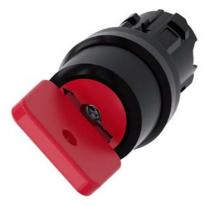
Key-operated switch O.M.R, 22 mm, round, plastic, lock number 73037, red, with 2 keys, 2 switch positions O-I, latching, actuating angle 90°, 10:30h/13:30h, Key removal O+I
