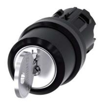
RONIS key-operated switch, 22 mm, round, plastic, lock number 455, with 2 keys, 3 switch positions I-O-II, latching, actuating angle 2x45°, 10:30h/12h/13:30h, Key removal I+O+II
