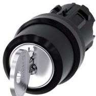
RONIS key-operated switch, 22 mm, round, plastic, lock number 455, with 2 keys, 3 switch positions I-O-II, latching, actuating angle  $2x45^{\circ}$ , 10:30h/12h/13:30h, Key removal O Z=50-unit packaging
