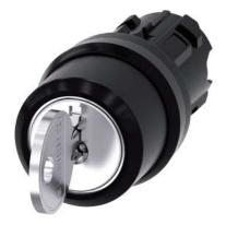
RONIS key-operated switch, 22 mm, round, plastic, lock number SB30, with 2 keys, 3 switch positions I-O<II, left latching, right momentary contact type, actuating angle 2x45°, 10:30h/12h/13:30h, key removal O+I, possible special locks: SB31, 421, 455
