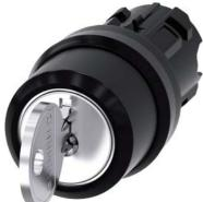
RONIS key-operated switch, 22 mm, round, plastic, lock number SB30, with 2 keys, 3 switch positions I-O<II, left latching, right momentary contact type, actuating angle 2x45°, 10:30h/12h/13:30h, key removal O, possible special locks: SB31, 421, 455
