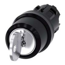
RONIS key-operated switch, 22 mm, round, plastic, lock number SB30, with 2 keys, 3 switch positions I-O-II, latching, actuating angle  $2x45^\circ$ , 10:30h/12h/13:30h, Key removal I+II, possible special locks: SB31, 421, 455
