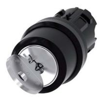
RONIS key-operated switch, 22 mm, round, plastic, lock number SB30, with 2 keys, 2 switch positions O-I, latching, actuating angle 90°, 10:30h/13:30h, key removal O, possible special locks: SB31, 421, 455, with laser labeling, upper case
