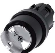
RONIS key-operated switch, 22 mm, round, plastic, lock number SB30, with 2 keys, 2 switch positions O<I, momentary contact type, Actuating angle 45°, 10:30h/12h, key removal O, possible special locks: SB31, 421, 455
