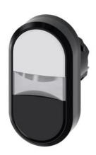
Twin pushbutton, 22 mm, round, plastic, white, black, pushbuttons, flat, with laser labeling, upper case and lower case, always upper case at the beginning of the word
