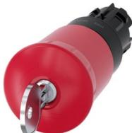
EMERGENCY STOP mushroom pushbutton, 22 mm, round, plastic, red, 40 mm, with lock Siemens, lock no. SMS1, positive latching, according to DIN EN ISO 13850, key-operated release
