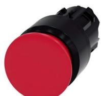
Mushroom pushbutton, 22 mm, round, plastic, red, 30 mm, latching, Pull-to-unlatch mechanism
