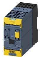
SIRIUS safety relay basic unit 3SK2 series 20 F-DI, 4 F-DQ, 2 DQ, 24 V DC Can be parameterized via SIRIUS Safety ES 45 mm width spring-loaded terminal (push-in) up to SIL 3 (IEC 62061) up to performance level e (ISO 13849-1) output expansions 3SK1, coupling relay 3RQ1 and fail-safe motor starters 3RM1 via device connector connectable
