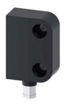
magnetically operated switch contact block rectangular small 26 x 36 mm, for left-hinged door, contacts: safety contacts 1 NO+1 NC, signaling contact 1 NC (31-32), with 8 mm latching connection plug 6-pole, without LED, the matching solenoid 3SE6714-3CA or offset by  $90^\circ$  3SE6724-3CA
