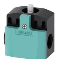
position switch plastic enclosure 50 mm, device connection 2 x (M20 x 1.5) 1 NO/1 NC integrated (not replaceable) quick-action contacts, rounded plunger
