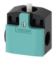
position switch with increased corrosion protection plastic enclosure 50 mm, device connection 2 x (M20 x 1.5) 1 NO/1 NC integrated (not replaceable) quick-action contacts, rounded plunger
