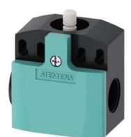
position switch plastic 50 mm increased corrosion protection device connection 2x (M20x 1.5) 1 NO/1 NC integrated (not replaceable) quick-action contacts, rounded plunger, functional at -40 °C shock and vibration test according to EN 61373, category 1B
