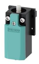
Position switch Plastic enclosure, 31 mm according to EN 50047 Control cabinet type 1 NO/1 NC snap-action contacts integrated (not replaceable) Rounded plunger Degree of protection IP40, with Self-sealing grommet Standard cover, turquoise With accessories: screws and mounting plate without locking sheet metal and seal
