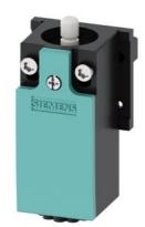
Position switch Plastic enclosure, 31 mm according to EN 50047 Control cabinet type 1 NO/1 NC snap-action contacts integrated (not replaceable) Rounded plunger Degree of protection IP40, with Self-sealing grommet Cover flat, turquoise With accessories: screws and mounting plate without locking sheet metal and seal
