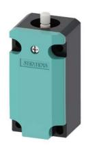
Basic switch with increased corrosion protection for position switch 3SE513 Enclosure plastic according to EN 50041 Device connection 1 x (M20 x 1.5) 2 NO/1 NC slow-action contacts without actuator head
