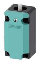
Basic switch for position switch 3SE513 Enclosure plastic according to EN 50041, 1 x (M20 x 1.5) 1 NO/1 NC quick action contacts without actuator head
