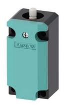
Basic switch with increased corrosion protection for position switch 3SE513 Enclosure plastic according to EN 50041 Device connection 1x (M20 x 1.5) 1 NO/1 NC quick action contacts without actuator head
