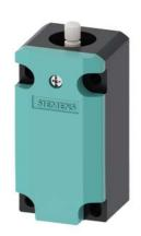
position switch basic switch plastic 40 mm according to EN 50041 increased corrosion protection device connection 1 x M20 x 1.5 1 NO/1 NC quick action contacts functional at -40  $^{\circ}$ C shock and vibration test according to DIN EN 61373, category 1B
