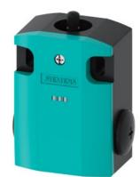
Basic switch for position switch 3SE51 Metal enclosure 56 mm wide Device connection 3 x (M20 x 1.5) 2 NO/1 NC slow-action contacts with 2 LEDs, yellow/green, 24 V DC without actuator head
