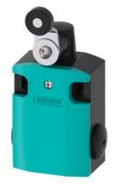
Position switch Metal enclosure 56 mm wide Device connection  $3x \, (M20x \, 1.5) \, 2 \, NO/1 \, NC$  slow-action contacts Rotary actuator right/left adjustable, with metal lever 27 mm long and plastic roller 19 mm
