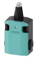
Position switch Metal enclosure 56 mm wide, Device connection 3x (M20x 1.5) 1 NO/1 NC quick action contacts, Roller plunger with 3 mm overtravel, Stainless steel roller 13 mm
