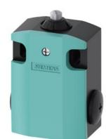
Position switch Metal enclosure 56 mm wide Device connection 3x (M20x 1.5) 1 NO/1 NC quick action contacts Plain plunger, stainless steel
