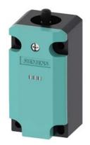
Basic switch for position switch 3SE51 Metal enclosure 40 mm according to EN 50041 Device connection 1x (M20 x 1.5) with 2 LEDs, yellow/green 24 V DC 1 NO/2 NC quick action contacts without actuator head
