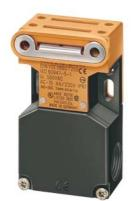
Safety position switch with separate actuator Molded-plastic enclosure lateral and face-end Slow-action contacts 1 NO+2 NC, 3 x (M20 x 1.5) Pull-out force 30 N Supplied without actuator
