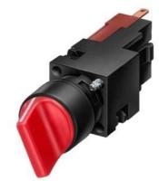
Selector switch, 16 mm, round, plastic, red, 3 switch positions I>O<II, momentary contact type, Retraction from left and right, Actuating angle 2 x 50 degree, 1 NO, 1 NO
