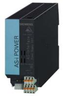
AS-i Power 2.6 A, max. 100 W 120 V/230 V AC AS-Interface power supply unit, IP20 IN: 120 V AC / 230 V OUT: AS-i, 2.6 A (30 V DC) Limitation of the output power max. 100 W, IP20 with integr. ground fault detection with AS-i data decoupling
