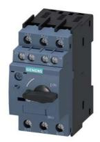
Circuit breaker size S0 for transformer protection A-release 18...25 A N-release 400 A screw terminal Standard switching capacity with transverse auxiliary switches 1 NO+1 NC
