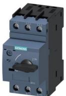
Circuit breaker size S0 For transformer protection A-release 4.5...6.3 A Shortcircuit release 130 A Screw terminal Standard switching capacity
