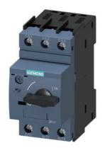
Circuit breaker size S0 For transformer protection A-release 3.5...5 A Short-circuit release 104 A Screw terminal Standard switching capacity
