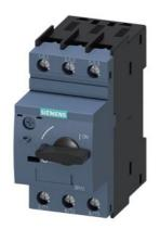
Circuit breaker size S0 For transformer protection A-release 0.7...1 A Short-circuit release 21 A Screw terminal Standard switching capacity
