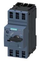
Circuit breaker size S00 for transformer protection A-release 9...12.5 A N-release 260 A Spring-type terminal Standard switching capacity
