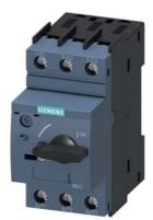
special type circuit breaker size S00 for transformer protection A-release 5.5...8 A short-circuit release 163 A screw terminal standard switching capacity ambient temperature -50  $^\circ$ C 500 switching cycles
