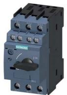
Circuit breaker size S00 for transformer protection A-release 4.5...6.3 A N release 130 A screw terminal Standard switching capacity with transverse auxiliary switches 1 NO+1 NC
