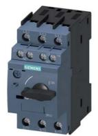
Circuit breaker size S00 for transformer protection A-release 2.2...3.2 A N release 65 A screw terminal Standard switching capacity with transverse auxiliary switches 1 NO+1 NC  $\,$
