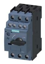
Circuit breaker size S00 for transformer protection A-release 0.45...0.63 A N-release 13 A screw terminal Standard switching capacity with transverse auxiliary switches 1 NO+1 NC
