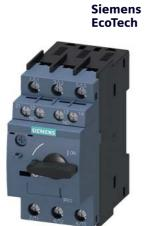
Circuit breaker size S00 for transformer protection A-release 0.18...0.25 A N-release 5.2 A screw terminal Standard switching capacity with transverse auxiliary switches 1 NO+1 NC
