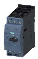
Circuit breaker size S2 for starter combination Rated current 65 A N-release 845 A screw terminal Standard switching capacity
