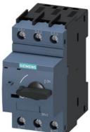
Circuit breaker size S0 for starter combination Rated current 32 A N-release 400 A screw terminal Standard switching capacity
