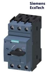
Circuit breaker size S00 for starter combination Rated current 5 A N release 65 A screw terminal Standard switching capacity
