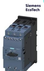
Circuit breaker size S3 for motor protection, CLASS 10 A-release 45...63 A N-release 819 A screw terminal Standard switching capacity with transverse auxiliary switches 1 NO+1 NC
