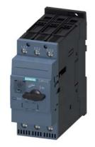
Circuit breaker size S2 for motor protection, CLASS 10 A-release 42...52 A N-release 741 A screw terminal increased switching capacity
