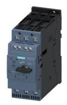
Circuit breaker size S2 for motor protection, CLASS 10 A-release 28...36 A N-release 520 A screw terminal increased switching capacity with transverse auxiliary switches 1 NO+1 NC
