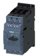
Special type Circuit breaker size S2 for motor protection, CLASS 10 A-release 35...45 A N-release 650 A screw terminal Standard switching capacity with transverse auxiliary switches 1 NO+1 NC Ambient temperature -50 °C 250 switching cycles
