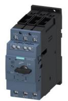
Circuit breaker size S2 for motor protection, CLASS 10 A-release 32...40 A N-release 585 A screw terminal Standard switching capacity with transverse auxiliary switches 1 NO+1 NC
